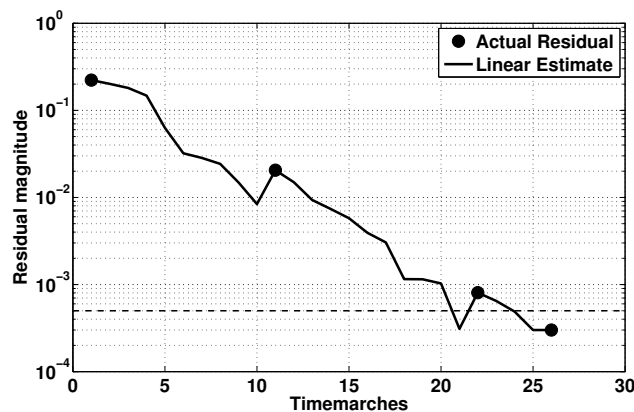
Figure 7.22: Typical convergence to a limit cycle in terms of the residual magnitude, \|\underline{x}(0) - \underline{x}(T)\|_2 , and number of timemarches. The dots are the residual values after each Newton step and the line is the estimated residual within the solution of each Newton step.
