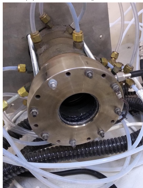
(b) Photo of the gas valve.
