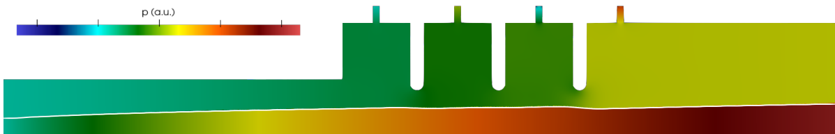
Figure 5.3 The pressure field in the gas valve. The white line shows the position of the aerogel. Darker / red colours shows higher pressure in the fluid, while bluer / lighter colours shows lower pressure in the fluid. The upper and lower sections separated by the aerogel line are equal at the reactor inlet on the left.
