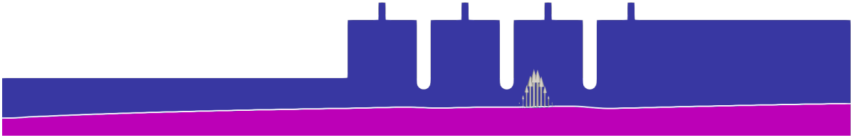
Figure 5.2 The 4-section gas valve configuration used to model the aerogel. The domain is split into two parts by the aerogel. The upper part (blue) and the lower part (pink) are solved independently, and the aerogel interface position is updated based on the resulting difference in pressure and shear force. The white arrows represents the magnitude of the weighting field belonging to one control point.
