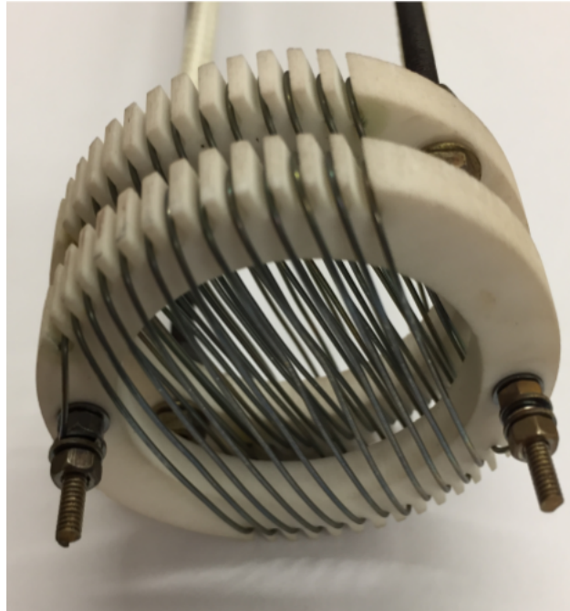
Fig. 2.2 Electric heater made up of 0.559 mm diameter Ni-Cr filaments wound between two parallel ceramic rings.
