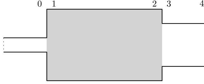
FIG. 18: A duct (highlighted in gray) with an area increase at the inlet and an area decrease at the outlet. The dotted lines represent other jumps or boundary conditions.
