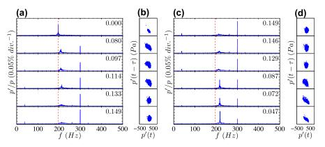
Fig. 5. Spectra (a and c) and Poincaré map (b and d) of pressure at a forcing frequency of 300 Hz ( $f_f/f_s = 1.54$ ) for various forcing amplitudes ( $A \equiv u'/u$ , indicated in plot). The forcing amplitude is first increased from a minimum to a maximum (a and b), and then it is decreased from that maximum to a similar minimum (c and d). The vertical dashed lines indicate the unforced self-excited frequency.
