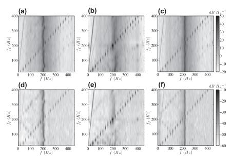
Fig. 3. PSD of pressure fluctuations (top row) and heat-release fluctuations (bottom row) at the start (left), middle (center), and end (right) of the forcing program. From left to right, the forcing amplitude goes from low, maximum, and then back to low as per Fig. 2.
