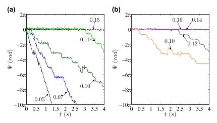
Fig. 6. Phase difference  $\Psi(t)$  at a forcing frequency of  $f_f = 220$  Hz ( $f_f/f_s = 1.13$ ) for increasing (a) and decreasing (b) forcing amplitudes ( $A \equiv u'/u$ , indicated in plot). For each A,  $\Psi(t = 0)$  is reset to zero in order to aid comparison of its temporal evolution.
