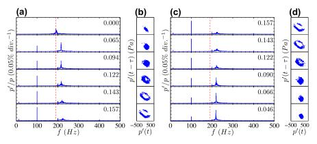
Fig. 4. Spectra (a and c) and Poincaré map (b and d) of pressure at a forcing frequency of 100 Hz ( $f_f/f_s = 0.51$ ) for various forcing amplitudes ( $A \equiv u'/u$ , indicated in plot). The forcing amplitude is first increased from a minimum to a maximum (a and b), and then it is decreased from that maximum to a similar minimum (c and d). The vertical dashed lines indicate the unforced self-excited frequency.
