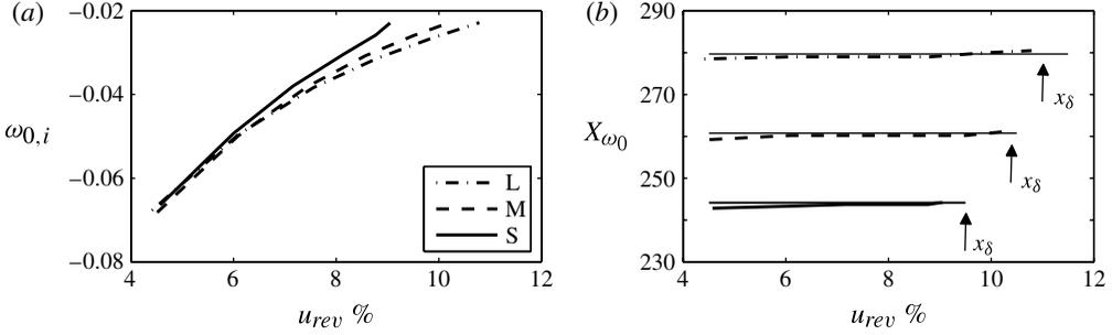
FIGURE 3. (a) Maximum absolute growth rate  $\omega_{0,i}$  and (b) corresponding streamwise coordinate  $X_{\omega_0}$ , as a function of the peak reversed flow  $u_{rev}$  %. The thin lines in (b) denote the location of the peak displacement thickness,  $\bar{\delta}_{max}$ .
