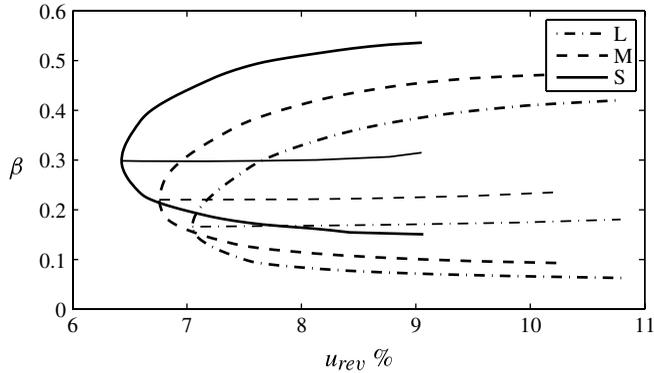
FIGURE 4. Neutral curves (thick lines) for the steady three-dimensional global mode, depending on the spanwise wavenumber  $\beta$  and the peak reversed flow  $u_{rev}$  %, for the three deceleration lengths. The thin lines correspond to the most amplified spanwise wavenumber.
