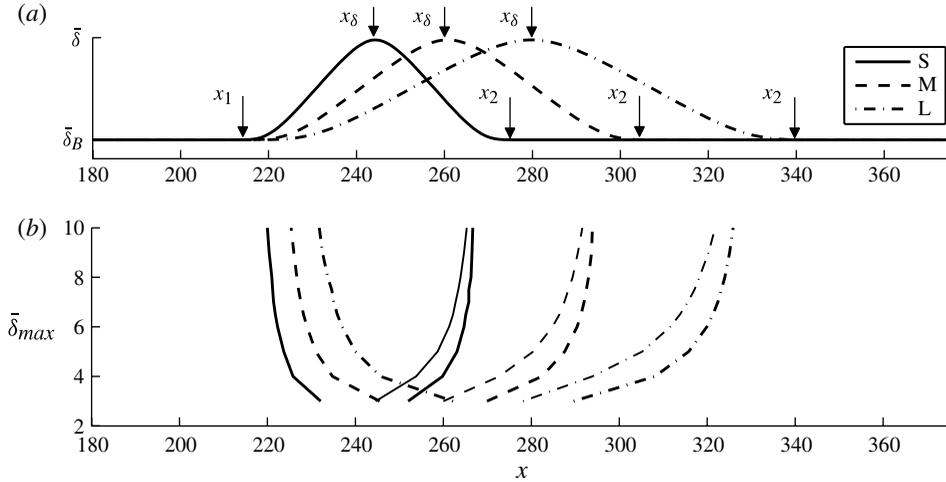
FIGURE 1. Laminar separation bubble models corresponding to cases S, M and L. (a) Transformed displacement thickness distribution  $\bar{\delta}$ . (b) Extent of the reversed flow region as a function of  $\bar{\delta}_{max}$ . Thick lines denote separation and reattachment lines and thin lines denote the location of the peak negative wall shear  $\tau_{min}$ .
