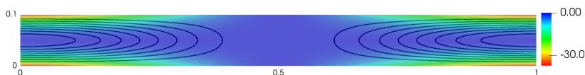
FIGURE 2. Spatial distribution of the decay rate production \sigma_\Omega in a flat channel. Black lines correspond to the oscillating flow velocity magnitude isolines \hat{u} = \text{const} .
