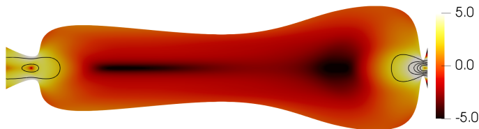
FIGURE 5. Spatial distribution of the absolute value of the decay rate production in the optimized channel (on a logarithmic scale), \ln(-\sigma_\Omega) . Black lines correspond to the oscillating flow velocity magnitude isolines \hat{u} = \text{const} .
