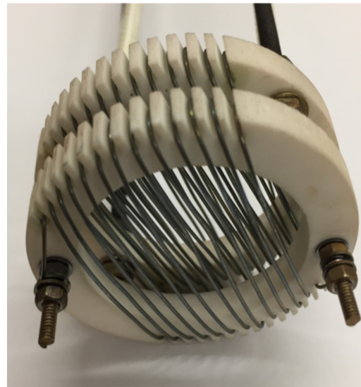
Fig. 2 Electric heater made up of 0.559 mm diameter Ni-Cr filaments wound between two parallel ceramic rings
