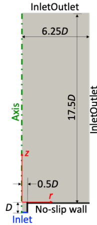
FIGURE 3: Domain used for RANS modelling of the turbulent jet flame. The blue box shows the region used to determine the likelihood of the RANS solutions against LES training data.
