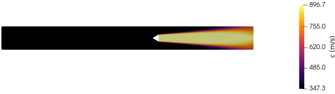
FIGURE 12: DISTRIBUTIONS OF THE SPEED OF SOUND c(x, y) IN THE THERMOACOUSTIC CALCULATION
