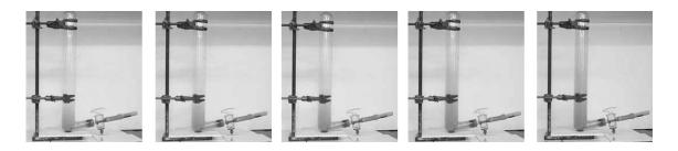
Boundary layers are caused by diffusion of momentum. This is a diffusion problem so if the fluid is initially stationary and the bottom plate starts moving at time t = 0, the thickness of the boundary layer increases in proportion to  $\sqrt{t}$ .
