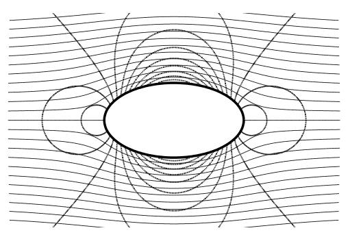
Viscous fluids obey the no slip condition. This means that a thin boundary layer forms around the surface of the ellipse, growing as the fluid moves from the front to the back. We will imagine for the moment that the boundary layer sticks to the surface all the way to the back of the ellipse.
