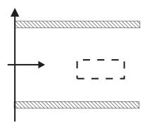
(a) Pressure pushes in the direction of the top plate's motion (*favourable* pressure gradient):
