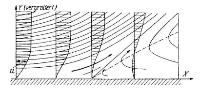
"A fluid layer which is set into rotation by friction at the wall pushes itself out into the free fluid where it causes a complete transformation of the motion."
