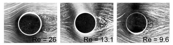
In aerodynamics, separation is usually undesirable because it increases drag, as we will see in chapter 8. It is usually impossible to change the fluid's viscosity but it is possible to delay separation in other ways, for example by injecting the momentum from the free stream flow directly into a boundary layer:
