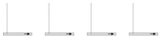
Film of a moving plate in a low viscosity fluid:
