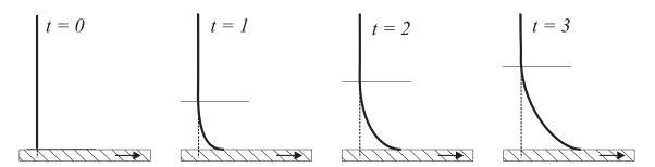
Similarly, if the fluid is moving at a constant velocity over a stationary flat plate, the thickness of the boundary layer increases in proportion to  $\sqrt{x}$ , where *x* is the distance from the front of the plate.
