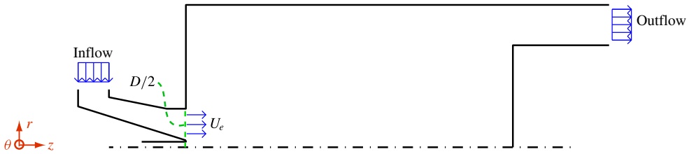
FIGURE 1. (Colour online) Illustration of the flow geometry. A cross-section in the axial-radial plane (constant azimuthal angle), showing the inflow (swirler inlet) and the outflow. The non-dimensional scales are shown: swirler outer diameter ( D ), and the exit velocity from the swirler ( U_e ). The coordinate system is also defined: the origin is at the centreline at the swirler exit location. The relative dimensions of the geometry are the same as in the numerical simulation, except that the numerical domain is longer in the downstream direction.
