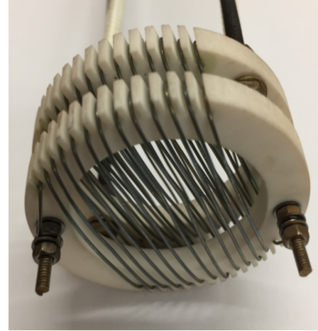
FIGURE 2: Electric heater made up of 0.559 mm diameter Ni-Cr filaments wound between two parallel ceramic rings.
